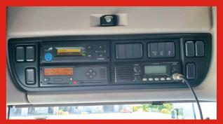
This one is under the roof. Each driver inserts a special card in it.
